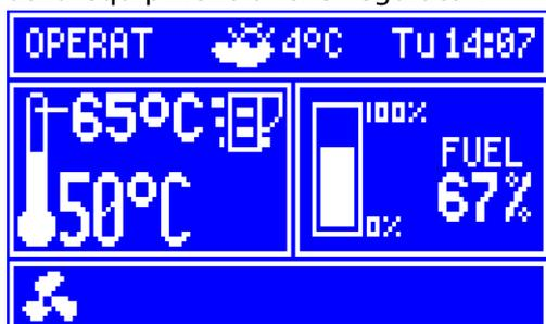
Fig. 18 Auxiliary window with fuel level gauge view.
